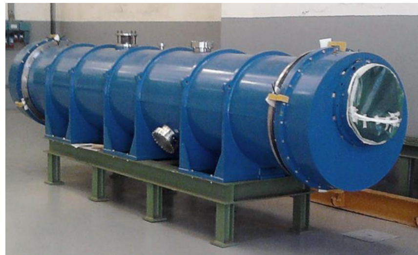
Full length curved, fast ramped s.c. SIS300 dipole magnet delivery: October 2013
