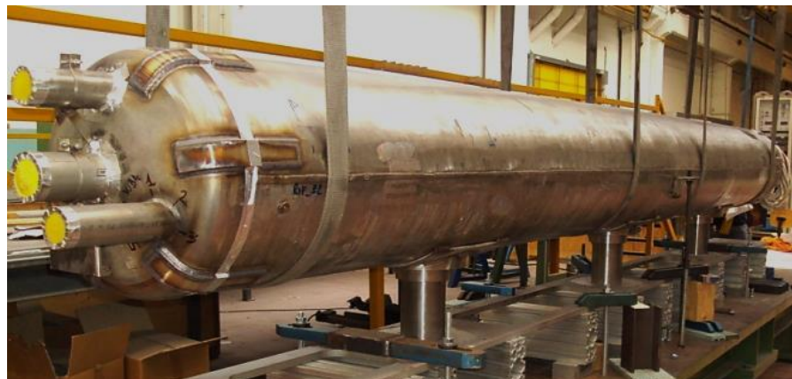
Full length curved, fast ramped s.c. SIS300 dipole magnet delivery: October 2013
