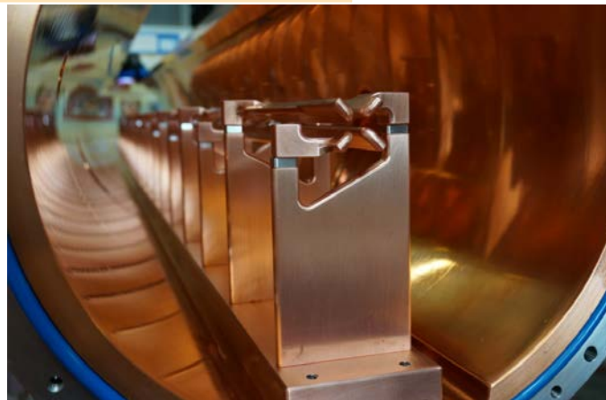
RFQ section installation in new hall
