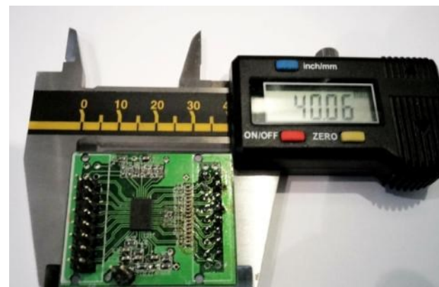
Readout Electronics developed for TPC, TOF, and ECAL (64 ch, 13-bit, 65 MS/PS)
