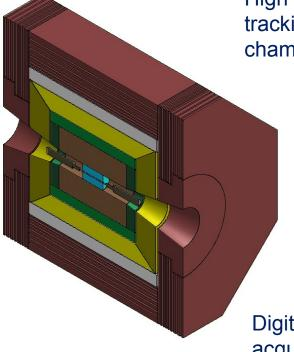
High precision charged-particle tracking (vertex detector+drift chamber)
