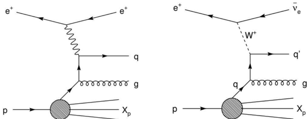
Examples of NLO diagrams of NC and CC. The current order of calculation is NNLO (2015).
