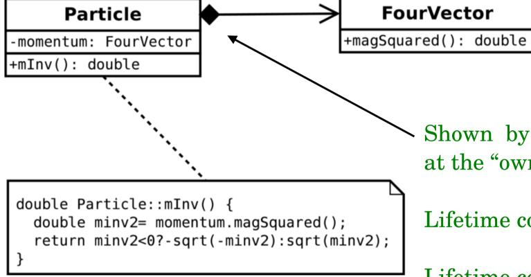
Lifetime control: construction and destruction controlled by "owner"
