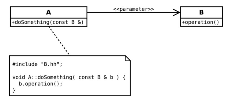
A depends upon B, because it uses B No data member of type B in A
