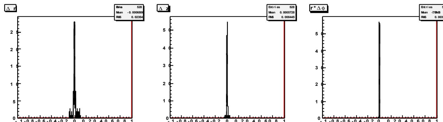
$$\begin{aligned}\Delta r &= 240 \text{ m}\mu \\ \Delta z &= 85 \text{ m}\mu \\ r\Delta\phi &= 40 \text{ m}\mu\end{aligned}$$
