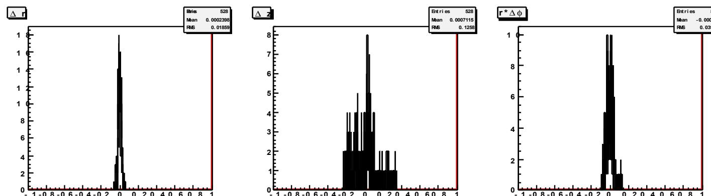
$$\begin{aligned}\Delta r &= 190 \text{ m}\mu \\ \Delta z &= 1.3 \text{ mm} \\ r\Delta\phi &= 400 \text{ m}\mu\end{aligned}$$
