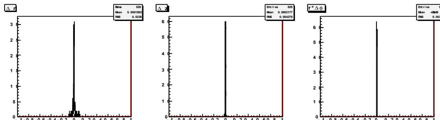
$$\begin{aligned}\Delta r &= 240 \text{ m}\mu \\ \Delta z &= 45 \text{ m}\mu \\ r\Delta\phi &= 30 \text{ m}\mu\end{aligned}$$
