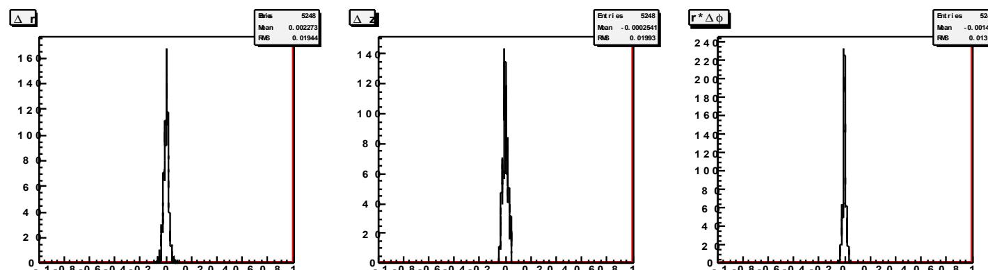
$$\begin{aligned}\Delta r &= 190 \text{ m}\mu \\ \Delta z &= 200 \text{ m}\mu \\ r\Delta\phi &= 130 \text{ m}\mu\end{aligned}$$
