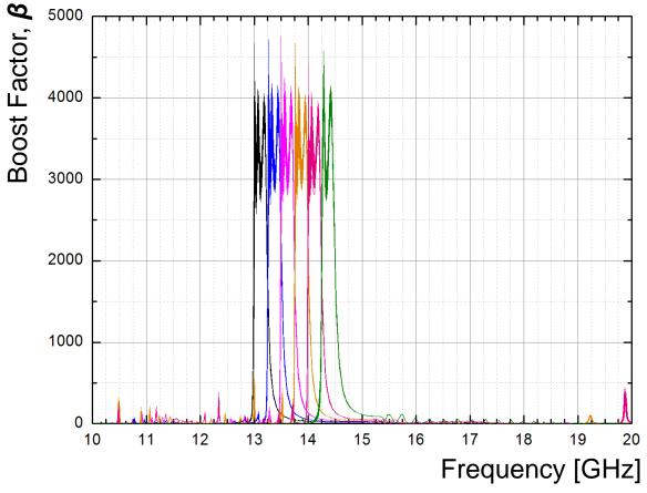
It is possible to adjust disc setting to reach sizeable  $\beta$  over broad bandwidth
