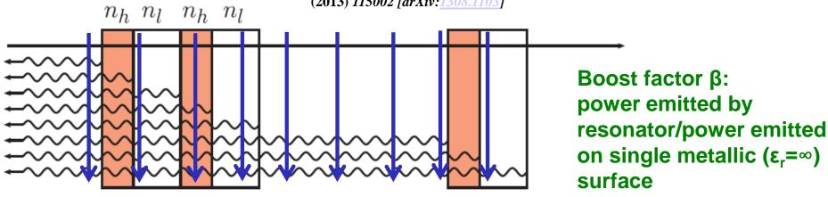
$(P/A)_{resonant cavity} \sim 2 \cdot 10^{-27} \text{ W/m}^2 \cdot (B_{\parallel}/10\text{T})^2 \cdot c_v^2 \cdot f(\epsilon_{m1}, \epsilon_{m2}) \cdot \beta$
