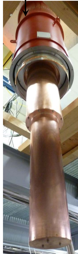
^3\text{He}/^4\text{He} Dilution Refrigerator
