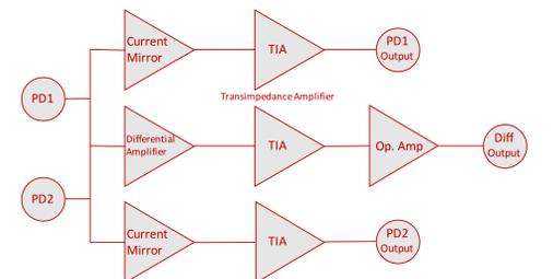
Figure 12. The scheme of the polarimeter board to generate DAVLL signal [4].
