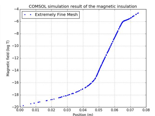
Figure 11. Magnetic field map from the circular guide to the shielding box.
