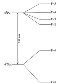
Figure 3. The Cesium  $D_2$ -transition energy level.
