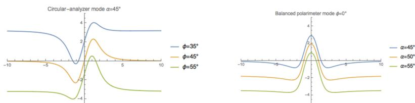
Figure 4. An expected signal of polarization rotation with respect to the frequency offset in a circular analyzer (left) and a balanced polarimeter (right) modes in unit dimensions. Both can be applied to lock the laser frequency [6].
