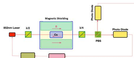
Figure 2. A schematic diagram of DAVLL system. The incident linear polarized laser into the Cs cell is rotated to have elliptical polarization if frequency was off from desired level.
