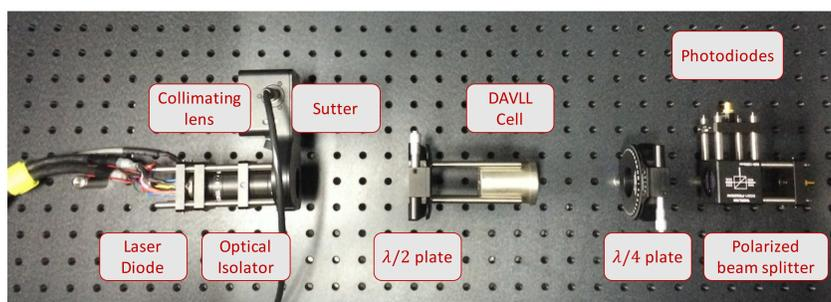
Figure 5. The experimental setup of DAVLL system.
