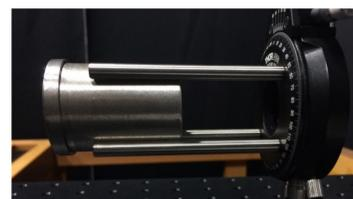
Figure 9. mu-metal shielding for Cs cell.
