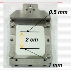
The surface roughness, the planarity of the target mounted in the holder and the sharpness of the apertures borders were careful monitored.
