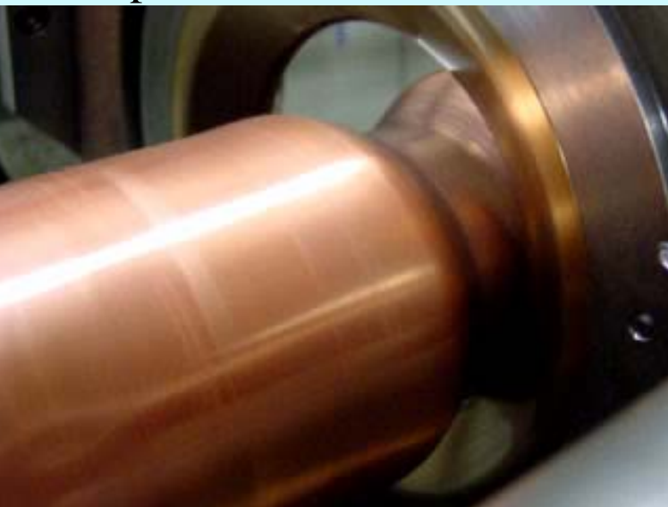
DESY Necking machine: new PC controlled necking procedure
