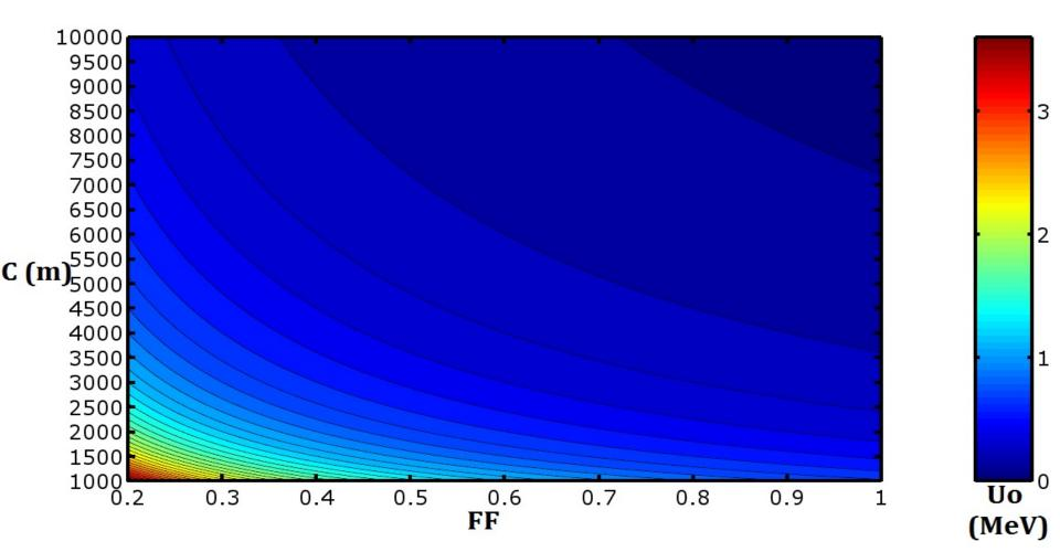
Scaling of Energy loss/turn with filling factor and circumference
