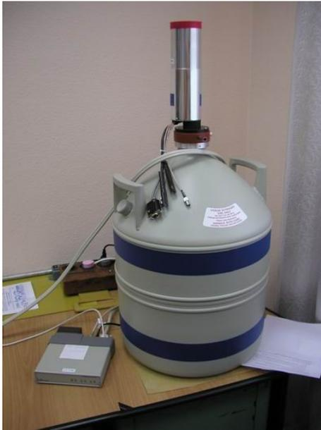
HPGe detector: energy resolution 1-2 keV at 1 MeV, photon energies up to 6 MeV (was used at VEPP-4M)
