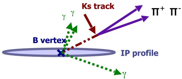
B decay point reconstruction from the  $K_S$  vertex, used in searches for NP right handed currents.
