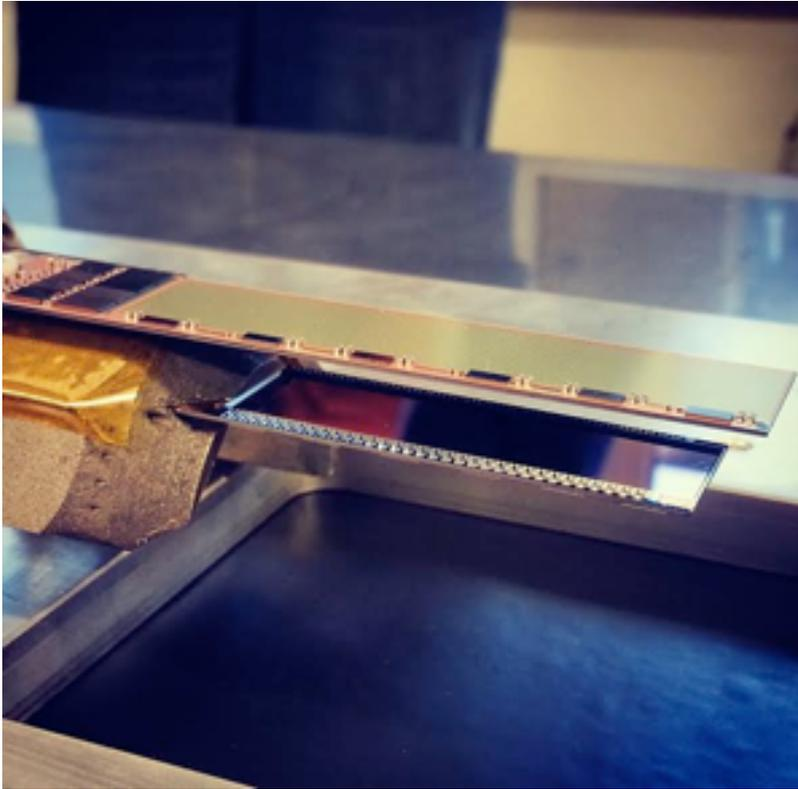
Test full-sized PXD modules in a beam. [Measure efficiency and S/N].
