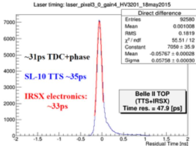
Production testing of readout with single photo-electron laser pulses in Hawaii; electronics resolution ~35ps
