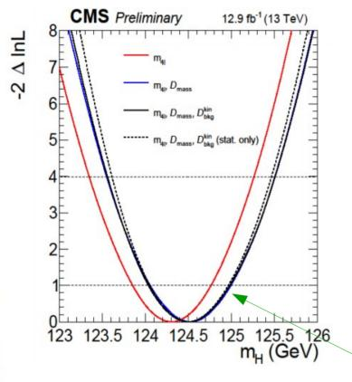
Using 4l 3D measurement, observed  $m_H = 124.50^{+0.48}_{-0.46}$  $(stat {}^{+0.47}_{-0.45}, syst {}^{+0.13}_{-0.11})$  GeV
