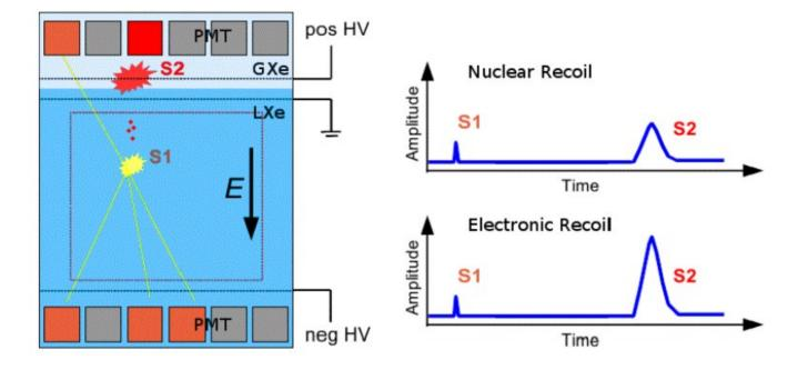
Scintillation light (S1) and ionization charge from primary event, which is converted to proportional scintillation (S2) in gas phase. Time between S1/S2 and top PMT pattern used to localize event. S2/S1 provides recoil discrimination.
