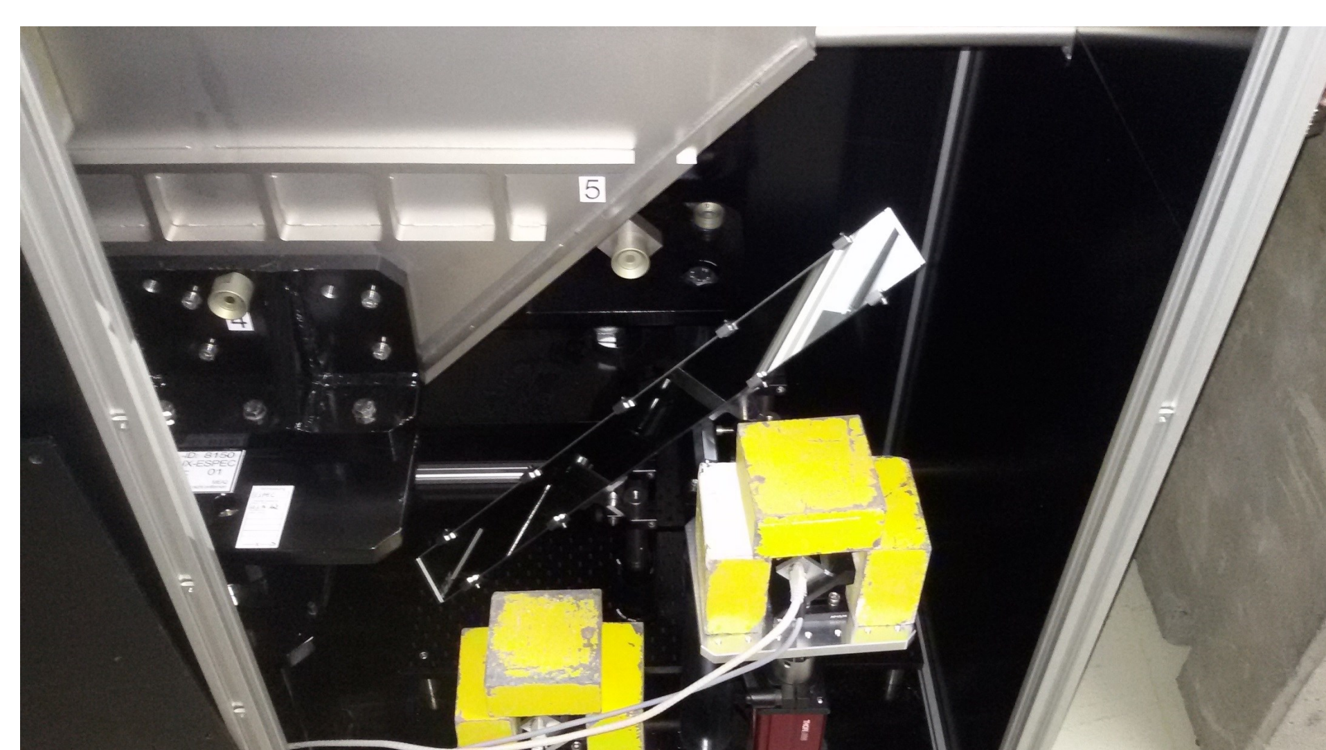
Two cameras looking on Lanex screen. A mirror is used to prevent radiational damage
