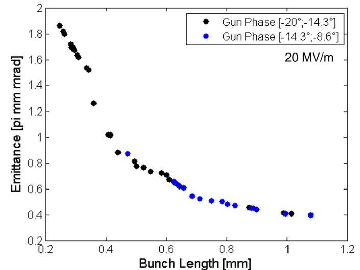
→ RF focusing at negative gun phases (relative to on crest phase)
