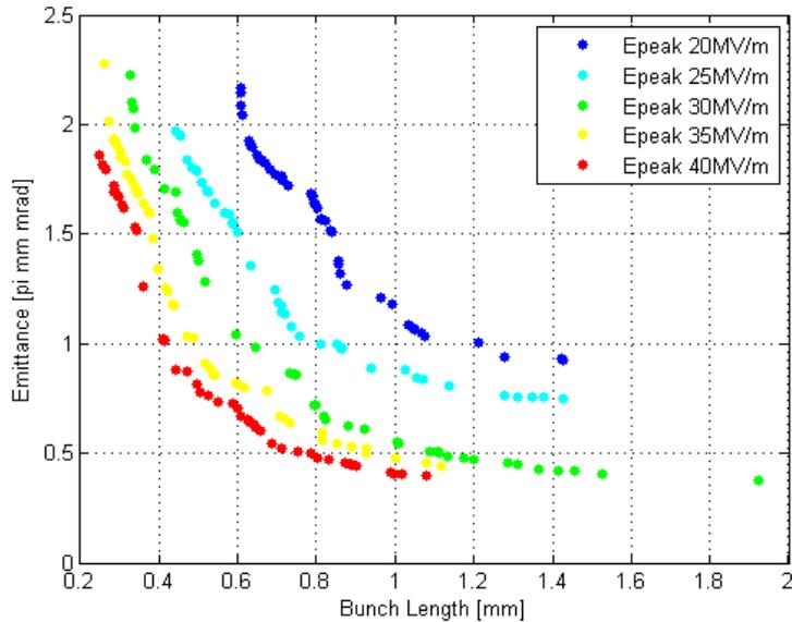
→ The lower limit of the Pareto optimum is given by the maximum gradient reached in the gun cavity (→ gun design)
