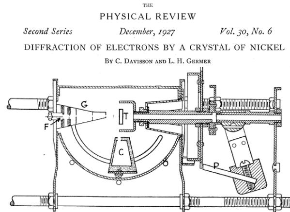
Fig. 2. Cross-sectional view of the experimental apparatus—glass bulb not shown.
