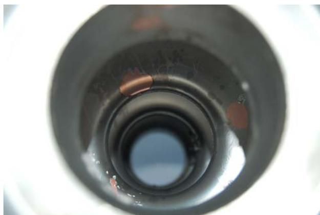
Fig. 7 Inner walls of dummy triple cavity after the deposition.
