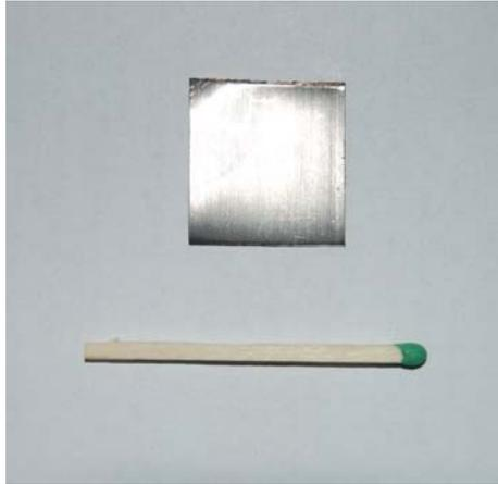
Fig. 6 Rough copper plate coated with Nb after HPWR at 80 bar.
