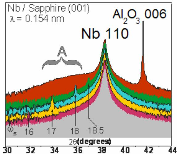
Fig. 7. Nb110 reflection measured for Nb/ sapphire film. The upper pattern represents results of symmetric  $\omega - 2\theta$  scan. Two components of peak profile are clearly seen. The other patterns were measured in detector scan for a fixed incidence angle showed in Figure.
