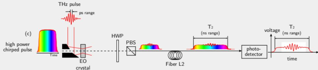
Balanced detection between the two polarizer ports: **Laser noise cancellation**
