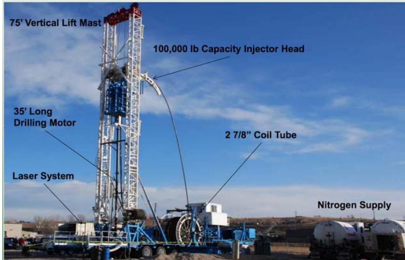
A portable oil-drilling setup includes a 20 kW fiber laser and a low-loss fiber-optic cable. The process potentially cuts the required power for drilling by nearly 90%.
