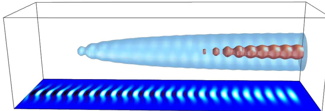
Beam self-modulates at plasma wavelength...
