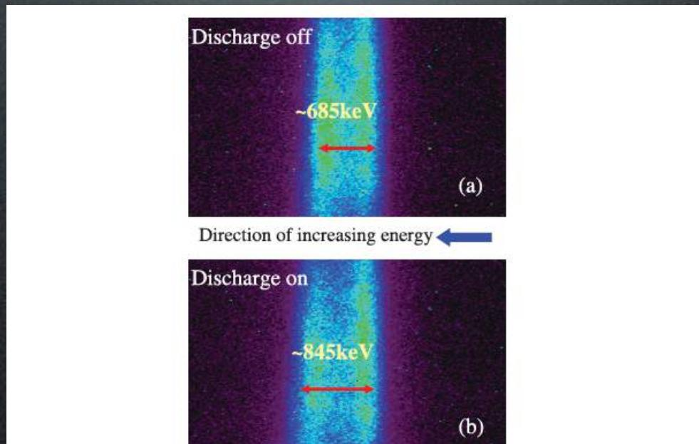
FIG. 3 (color). Raw video images from the electron energy spectrometer. Energy dispersion is in the horizontal direction. (a) Discharge is off in the PASER cell. (b) Discharge is on in the PASER cell. In both cases,  $\sim 1.5\%$  peak-to-peak energy modulation was imparted.
