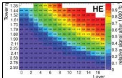
Predicted HCAL Endcap signal response after 1000fb<sup>-1</sup> versus active layer and  $\eta$
