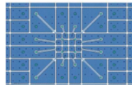
Fig. 8. Layout of 50  $\mu\text{m} \times 50 \mu\text{m}$  pixel cells surrounded by larger cells to be compatible with the PSI46dig readout chip.
