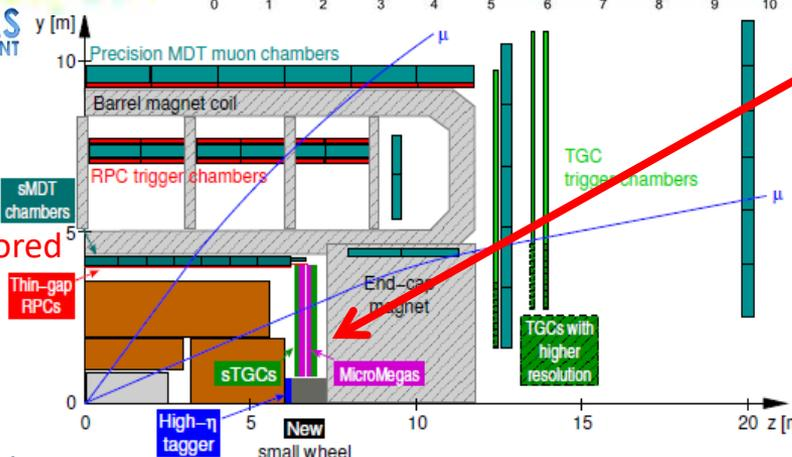
**ATLAS: improve endcap muon tracking and trigger**
