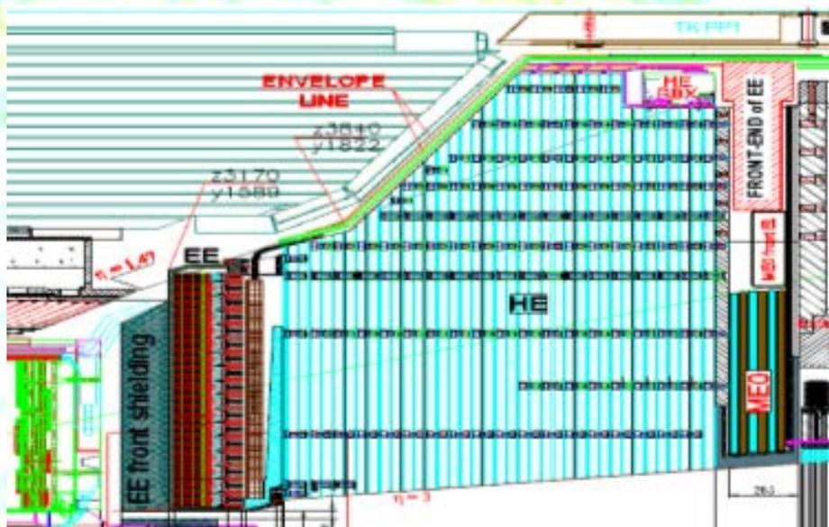
**CMS scintillator-based HCAL with 30% of volume replaced by finger tiles to reduce optical path and attenuation**
