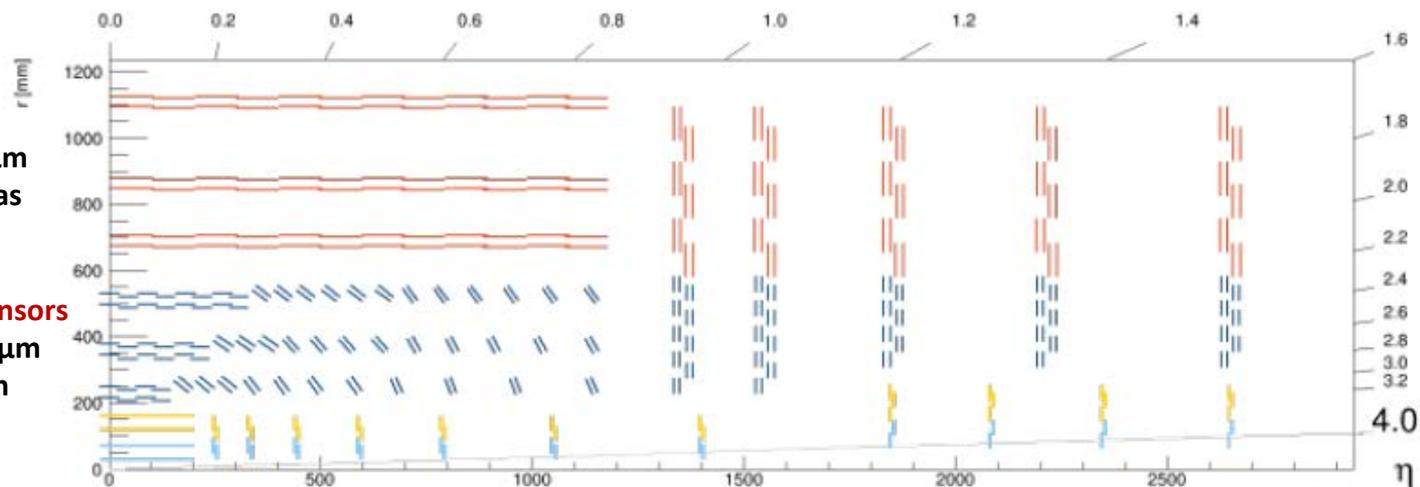
**HL-LHC (3000fb<sup>-1</sup>) implies doses up to 2×10<sup>16</sup>n<sub>eq</sub>/cm<sup>2</sup> and 1Grad (also up to 200 collisions per beam crossing). However n-in-n, n-in-p planar, 3D and diamond sensors are useable after such doses**
