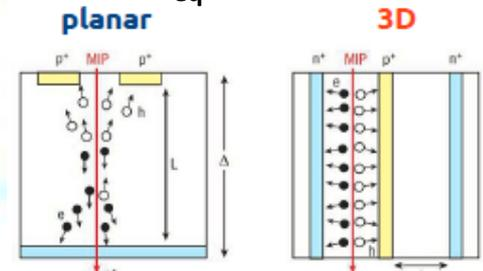
(3D sensors installed in ATLAS IBL)
