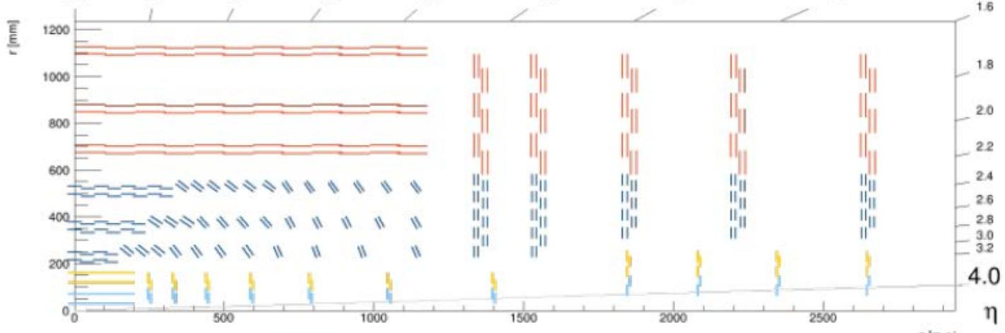
Paired layers with short strips (outer radii) and long pixels plus short strips (inner radii)
