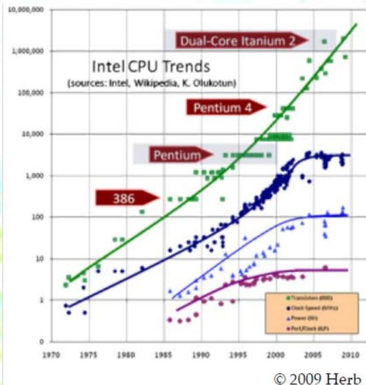
The available transistors are used for **adding new CPU cores** while keeping the clock frequency basically constant, thus limiting the power consumption
