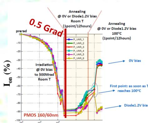
Significant  $V_t$  shift can develop with annealing depending on Temperature, Time, Bias, Device type, L, W, Received dose, but Indication that detrimental effects can be "avoided"/delayed by keeping cold
