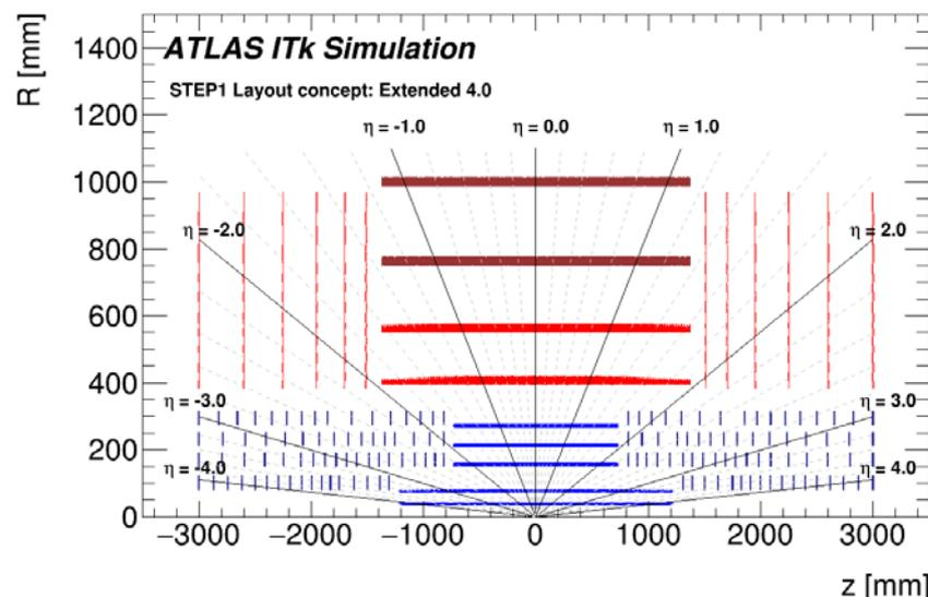
Several layouts are under consideration including (not shown here) pixel layers with inclined sensors. The main differences in the ATLAS Phase-II Upgrade Scoping Document (CERN-LHCC-2015-020 ; LHCC-G-166) were in terms of the  $\eta$  coverage of the tracker which relates to the area of the pixel system ranging from  $\sim 13\text{m}^2$  to  $\sim 16\text{m}^2$ .
