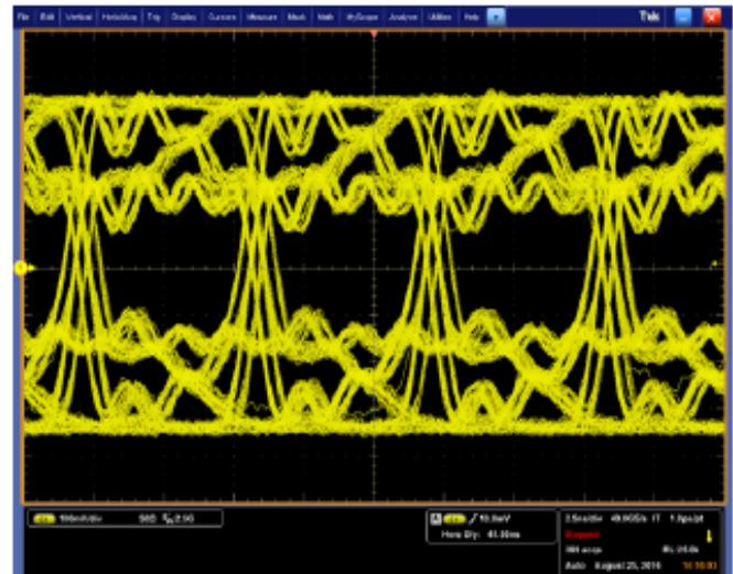
Eye diagram for PRBS-31 (equivalent to no data encoding) for 160 Mbps and double the capacitive loads
