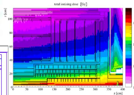
Strip detectors must survive damage to lattice equivalent to that from  $1.2 \times 10^{15}/\text{cm}^2$  1 MeV neutrons and 0.5 MGy (Pixels >  $\times 10$  this)
