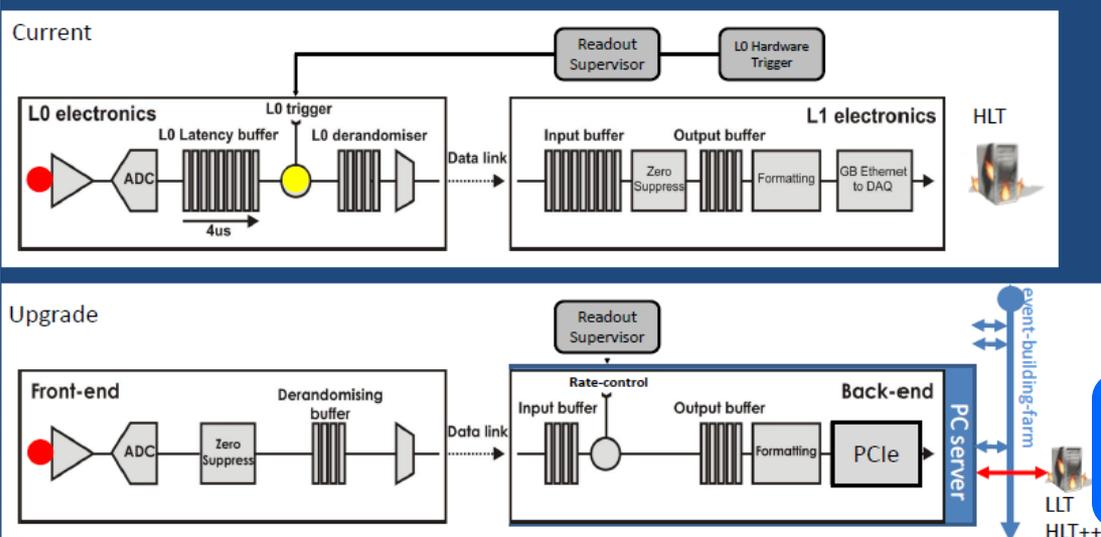
Data compression on Front-end driven by link cost:
