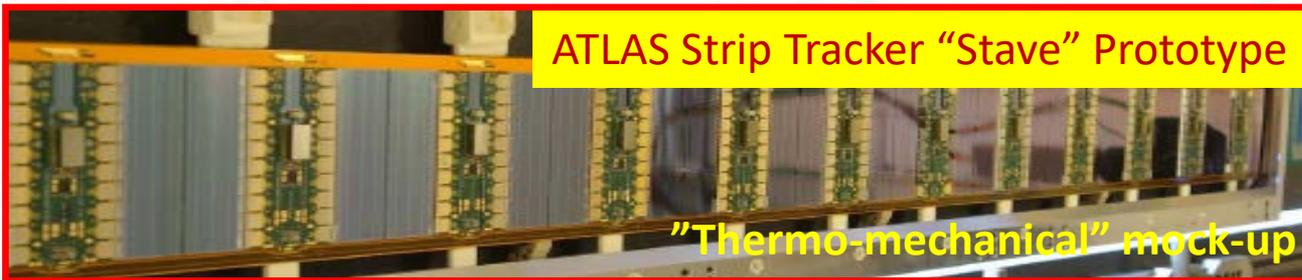
Single-sided modules sandwiched around low mass structures
