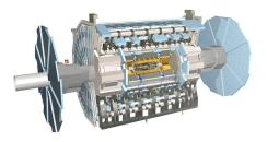
ATLAS Emphasis on jet and missing  $E_T$  resolution, particle identification and standalone muon measurement
