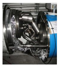
On September 19, 2008 one superconductor joint failed, damaged the vaccum enclosure, caused a catastrophic release of Helium and collatoral damage (up to 50 cm displacement of several quadrupoles, beam pipe contaminated with soot, ...)
