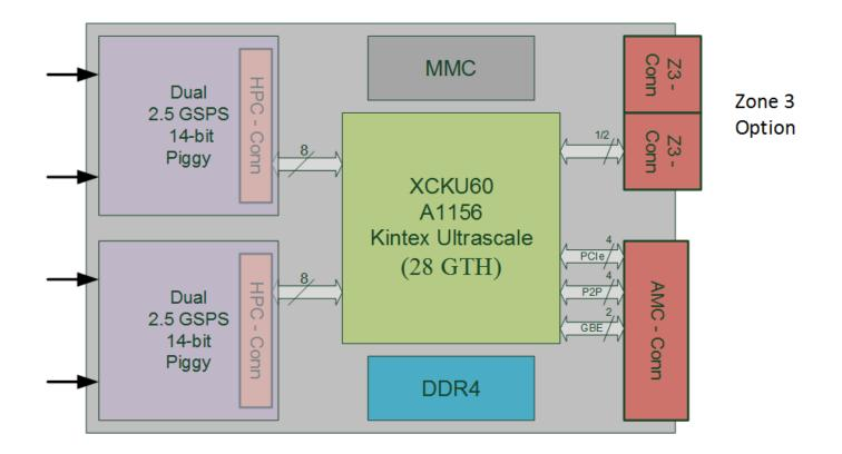
Same carrier can be used for 8 channel 14/16-bit GSPS design FMC or custom tbd.
