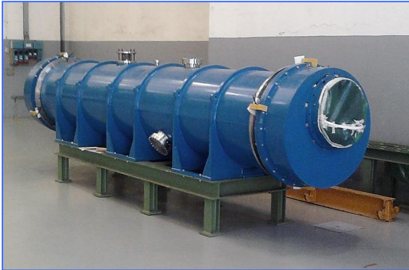
Fastest ramped, full size s.c. \cos(\theta) dipole magnet world wide (SIS300 prototype)
