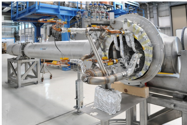
First cryogenic bypass line delivered and under cold testing at GSI (Poland)
