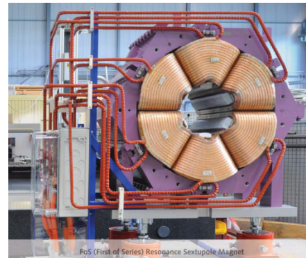
FoS (First of Series) Resonance Sextupole Magnet
