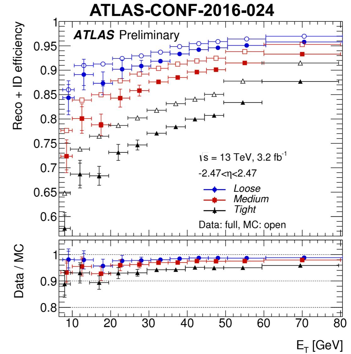
Detector performance well understood, data used to correct simulation.
