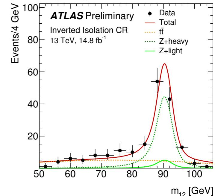
Reducible background from Z+jets and  $t\bar{t}$  estimated using data-driven methods
