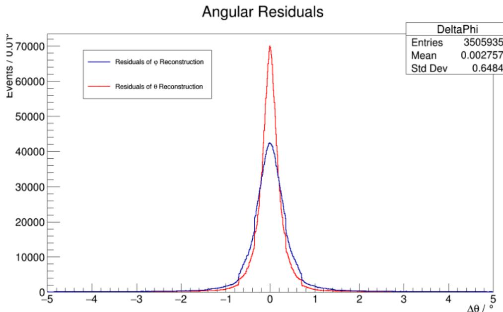
High and uniform reconstruction efficiency of  $\varphi$  over the whole azimuthal angle
