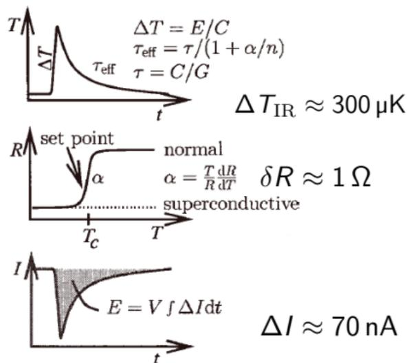
Figure: Sketch of TES characteristics [de Korte et al. (2003), Proc. SPIE 4851].
