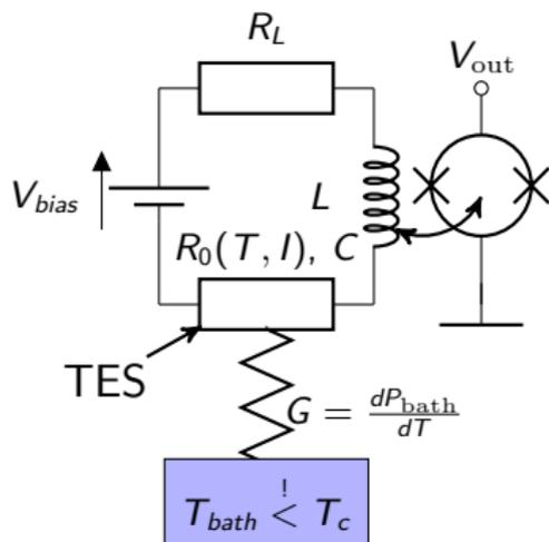
Figure: TES readout circuit.
