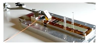
The modules will be tested again to ensure that the kapton attachment was successful (no shorts, no cracks introduced).
