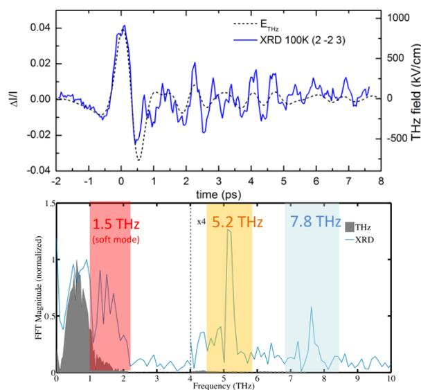
Figure 1: upper panel: X-ray diffraction intensity change of (2 -2 3) Bragg peak in SrTiO<sub>3</sub> at 100K (blue) overlaid with the THz pump electric field (dotted line). Lower panel: Fourier transform reveals energy transfer from the low frequency soft mode phonon at 1.5 THz into the higher phonon modes at 5.2 and 7.8 THz through nonlinear phonon dynamics mediated by the large anharmonicity of the soft mode potential.
