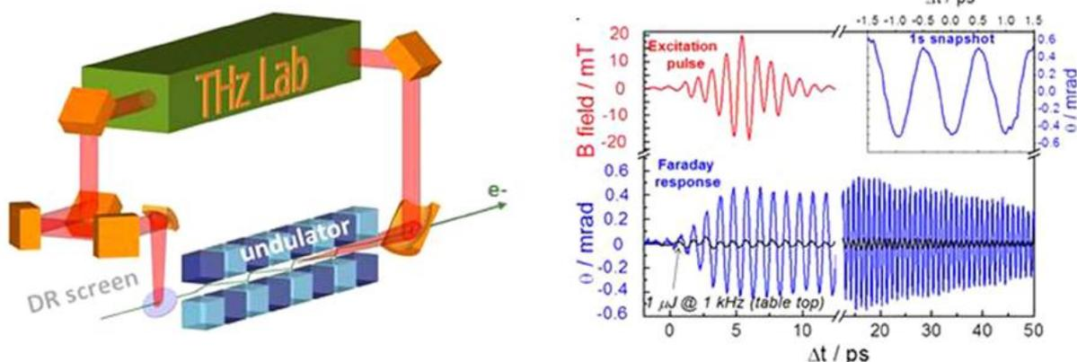
Figure: Arrangement of the superradiant THz sources at TELBE (left) and transient Faraday measurement of a selectively excited spin wave in NiO [1]. Note that the 2 THz sources (diffraction radiator – single cycle and undulator – multi cycle) can be operated in parallel without any observable degradation of the THz pulse properties.
