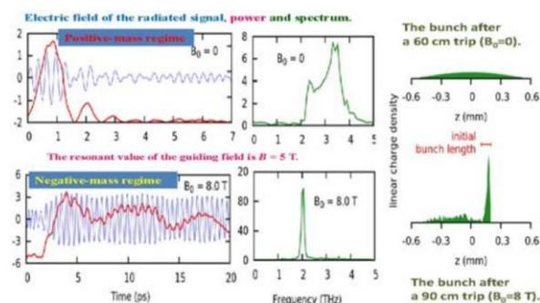
One can propose a design in which the electron bunch with the particles energy of 5.5 MeV (mass factor of 12) scatters the undulator field with a period of 2.5 cm into the wave with a frequency of about 2 THz. The negative mass regime is realized at the axial field from the range near 8 T and the undulator field amplitude of about 0.2 T. The efficiency of this process (the share of the initial electron energy passed to the radiated wave) can be as high as 20%.
