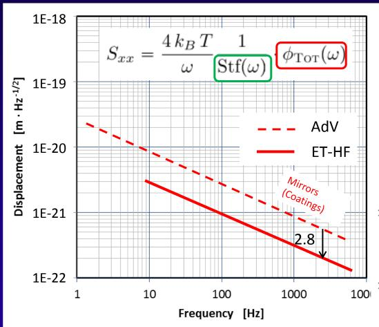
Coating thermal noise is dominant around 100 Hz where the detectors are more sensitive
