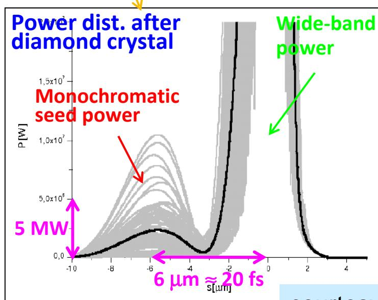
Self-seeding of 1-μm e<sup>-</sup> pulse at 1.5 Å yields **10<sup>-4</sup> BW** with low charge mode
