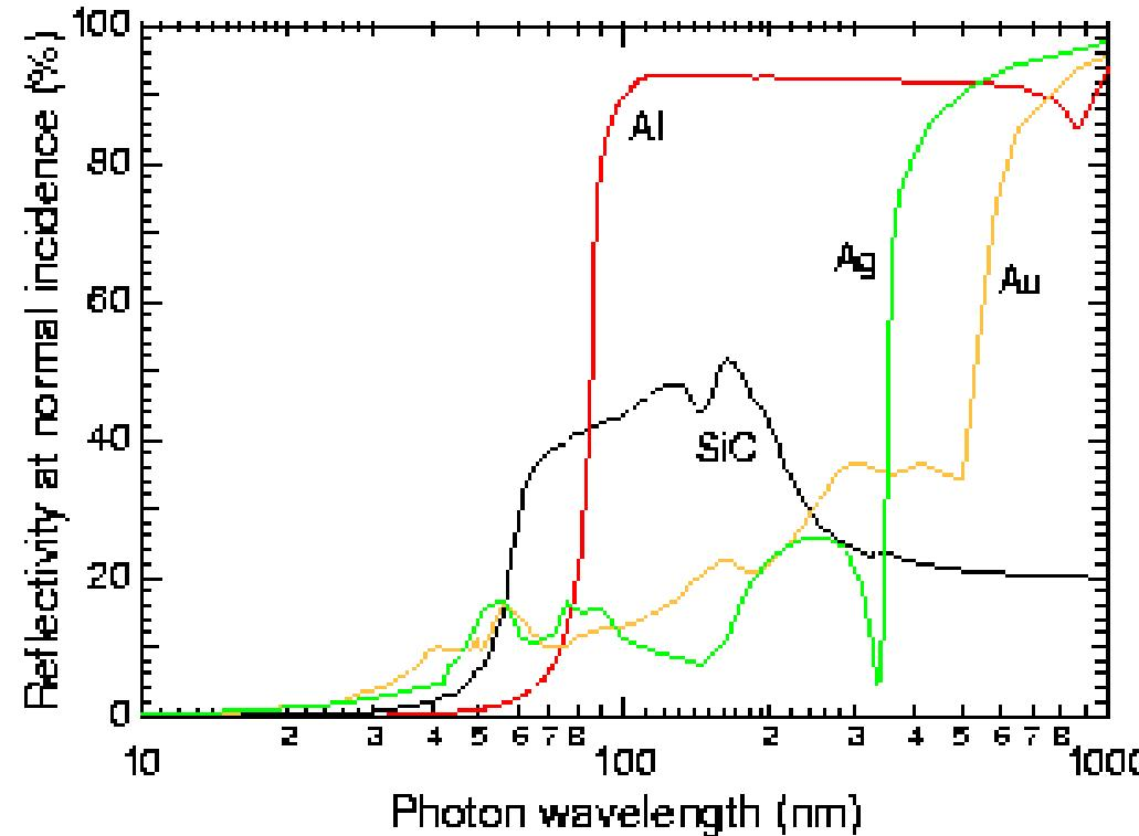
Reflectivity of most surfaces at normal incidence drops drastically at wavelengths below 100 – 200 nm.
