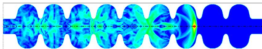
Wake field: trailing particles lose energy w.r.t. head of bunch !
