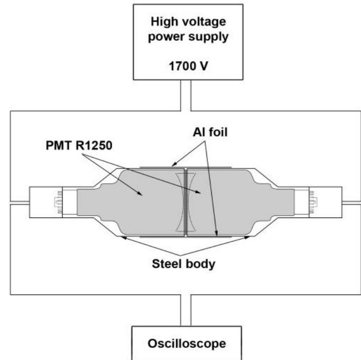
Coincident noise pulses in **face-to-face optically coupled PMTs**.
