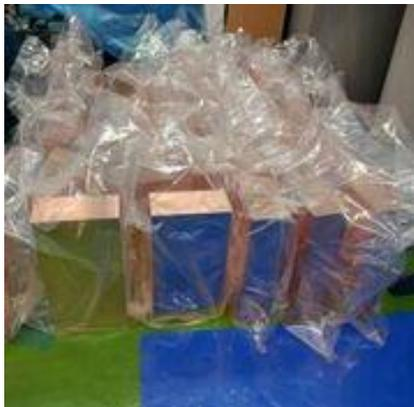
This year I purchased **600kg** of copper at **Mitsubishi Materials** specially melted for us only. Freshly manufactured (**1.5month or less old**) electroformed copper sheets were used to avoid  $^{60}\text{Co}$ . Cu bars were cut into standard size bricks, surface milling, and cleaning according to the Majorana procedure was done. The HPGe measurements found **no  $^{60}\text{Co}$  access** (UL 0.2mBq/kg at 90%CL).
