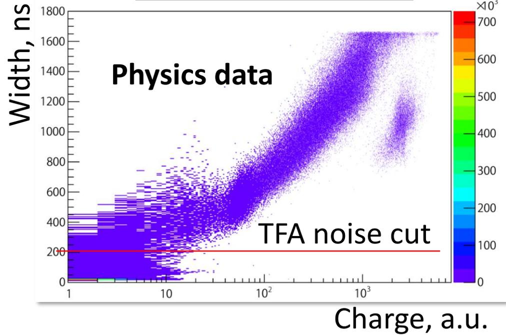
PMT noise >99.9% of data, from single to several narrow pulses (trains) was effectively cut by TFA.
