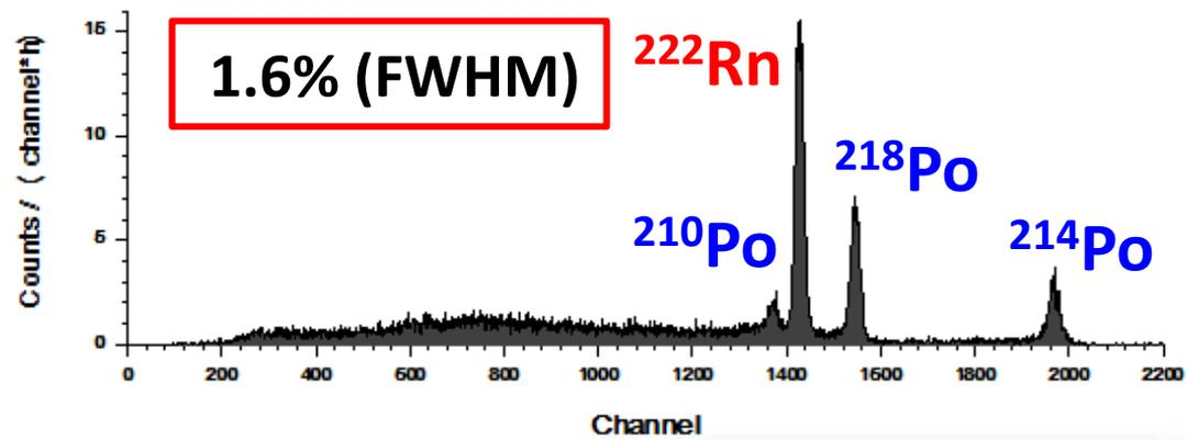
Direct detection of the Radon  $\alpha$ -decay in the air.
