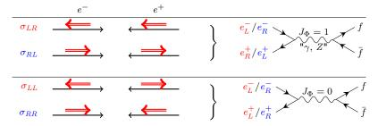
▶ For a bunch of particles the polarization *P* is defined as:
