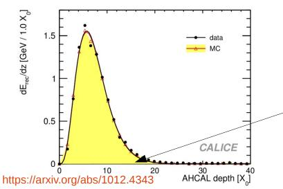
Longitudinal Profile of 10 GeV positron In Fe:  $X_0 = 1.757 \text{ cm} (\lambda = 16.77 \text{ cm})$ Fully equipped part of the prototype ~ 15  $X_0$ (~26 cm of steel)
