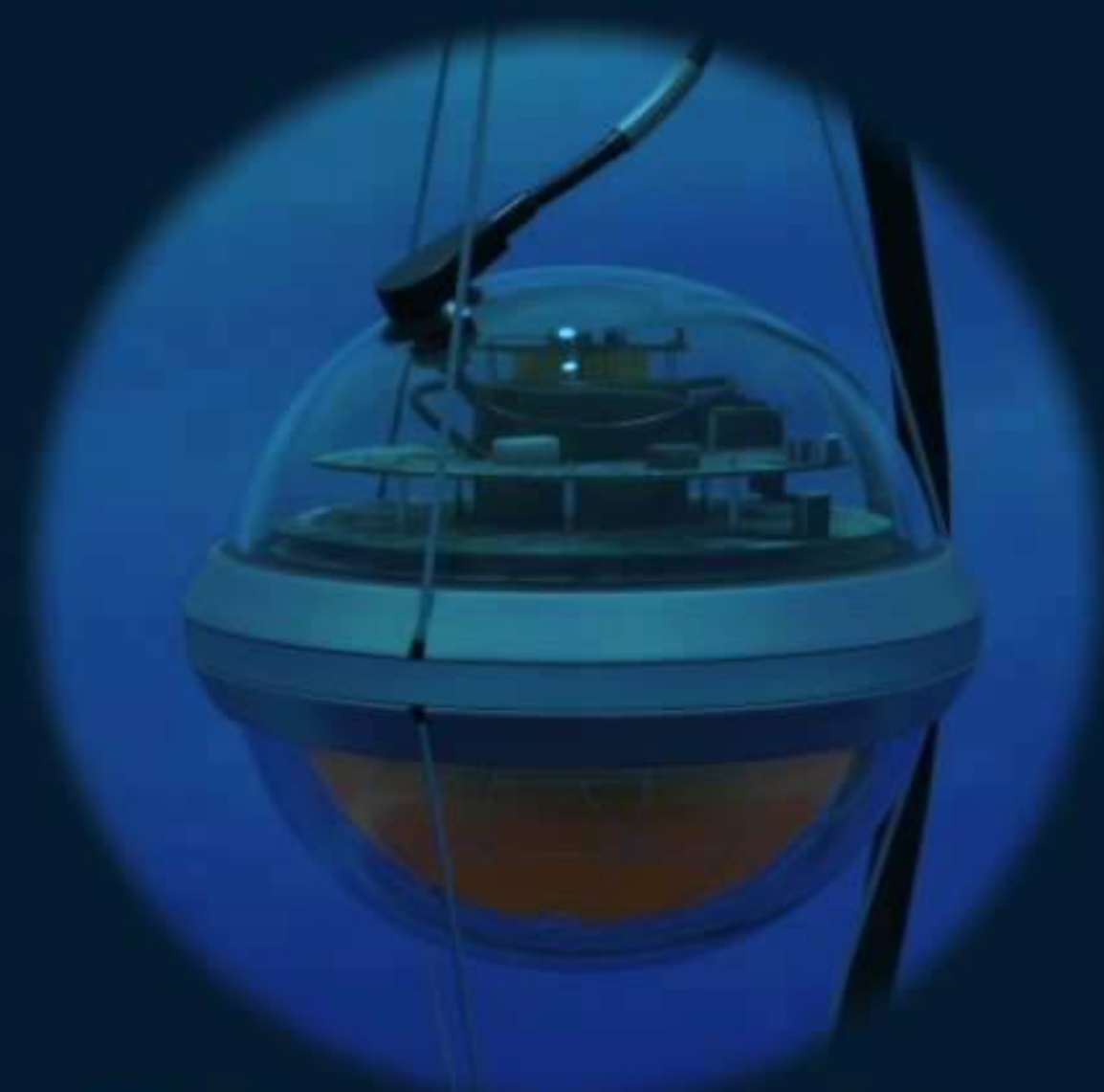
Digital Optical Module DOM 86 strings 5160 optical sensors
