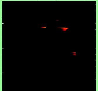
no emission @ 120MV/m 5 emitters @ 150MV/m ↓ best EP/HPR sample yet
