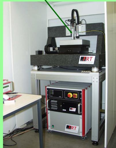
combined with atomic force microscope AFM Scanning speed: (100×100) pixels in 1 min
