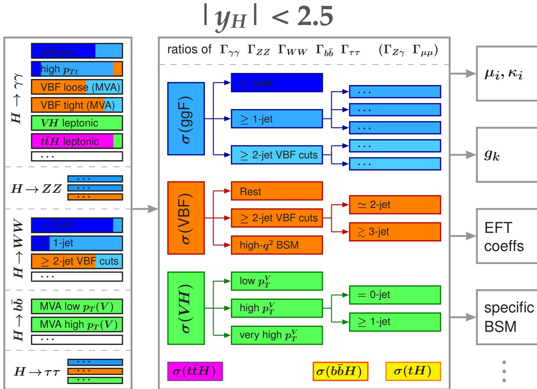
**Simplified template cross sections (STXS)** provide a natural evolution of Run-1 style signal strength measurements
