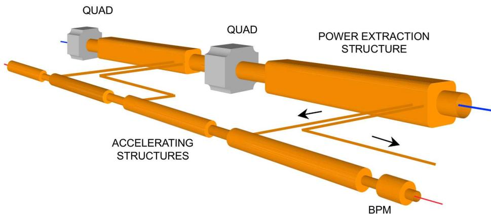
Figure 3: Principle of two-beam acceleration: as the high-current drive beam travels through the Power Extraction Structure the wakefield is coupled into the accelerating structures of the main beam.
