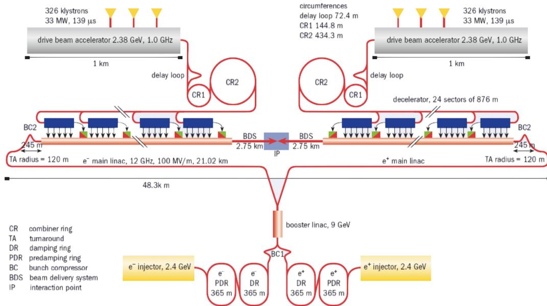
Figure 2: The layout of the Compact Linear Collider for operation at 3 TeV. The lower part shows the generation of the high-energy beam; the upper part describes the generation of drive beams.
