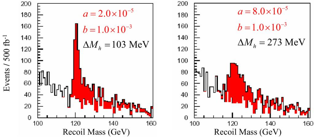
Figure 1: The Higgs boson recoil mass spectrum for two assumed resolutions for decays  $e^+e^- \rightarrow ZH$ , where the  $Z$  decays into 2 muons. The quantities  $a$  and  $b$  refer to the terms in the transverse momentum resolution  $\sigma p_t/p_t = ap_t \oplus b/\sin\theta$  (from ref, [6])
