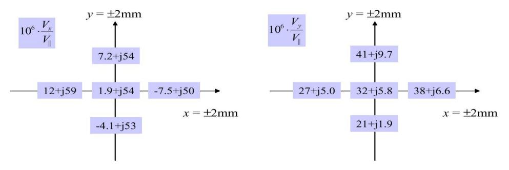
Xy-dependence: data only for DESY-downstream-coupler
