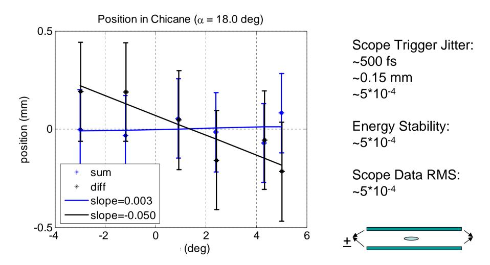
~5 mm orbit change in ACC1 causes 5 degree tilt of beam ? causes 200 um BPM error 100 um orbit jitter in ACC1 causes small tilt of beam causes 4 um BPM error
