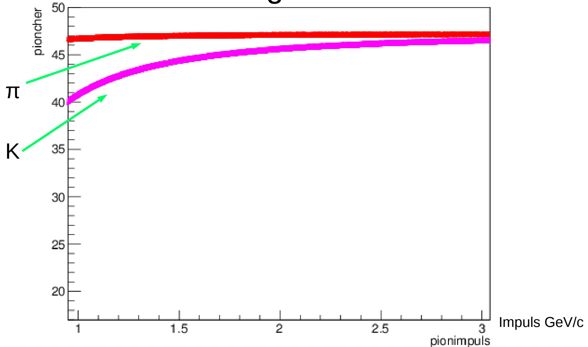
The Cherenkov photon angle inside our radiator fused silica( $n \sim 1.47$ ) for kaons and pions
