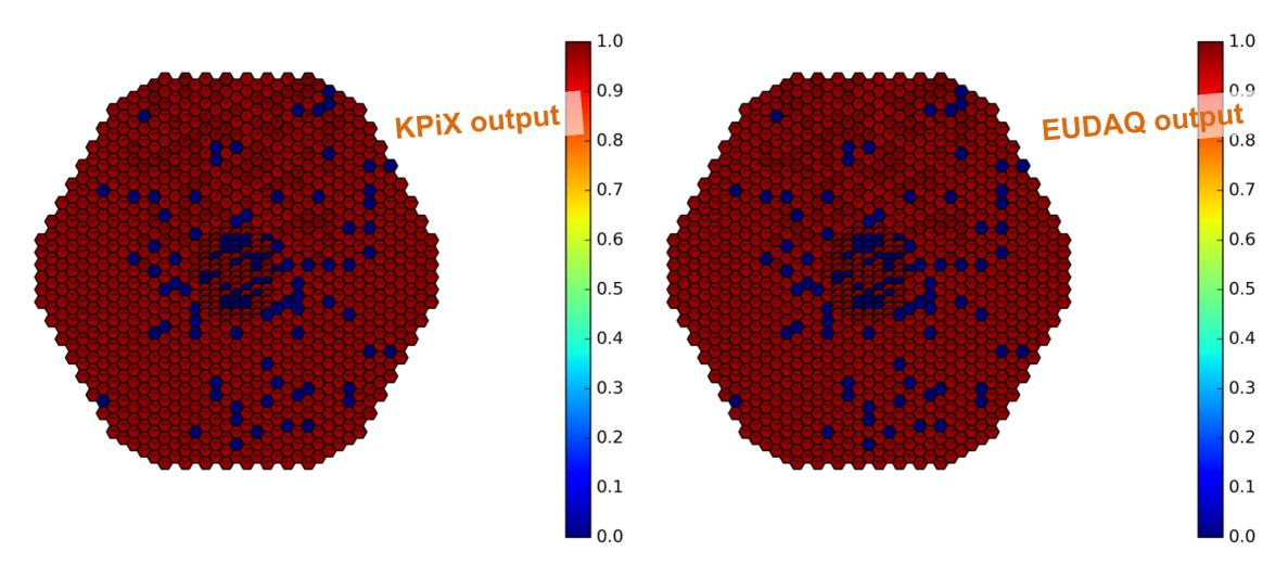
\* event mapping on the ECal sensor for KPiX tests at DESY
