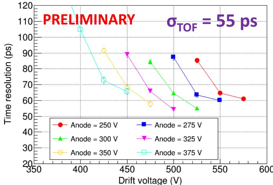
A 5 mm MgF<sub>2</sub> + 10 nm Al photocathode showed in last beam a time resolution of **55 ps** and **~2.6 phe/muon**.
