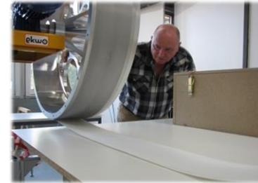
4. **Foil lamination** with black 25  $\mu\text{m}$  thick capton foil (both sides, ensures light tightness) and **end piece gluing**
