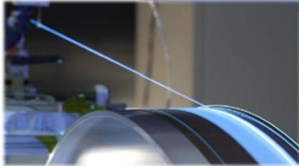
2. **Glue curing** with wheel rotating for 12h in an area with controlled humidity and temperature
