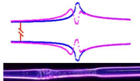
Fiber Bumps larger than 500 µm must be cut away and the fibre re-glued (~15 min, 1-2×/spool).
