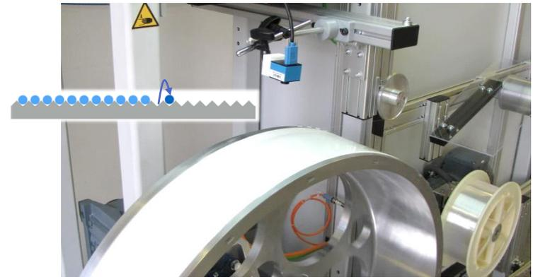
Alignment pin groove in the wheel, filled with glue during winding, allows precision positioning at later production steps
