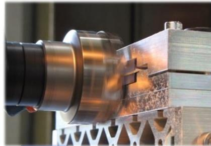
5. **Optical cut** with a milling machine (polishing with a diamond head)
