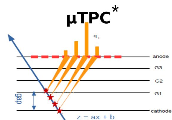
Use the drift gap as a “*micro time projection chamber*” and reconstruct the position of **each primary ionization** by the electron drift velocity
