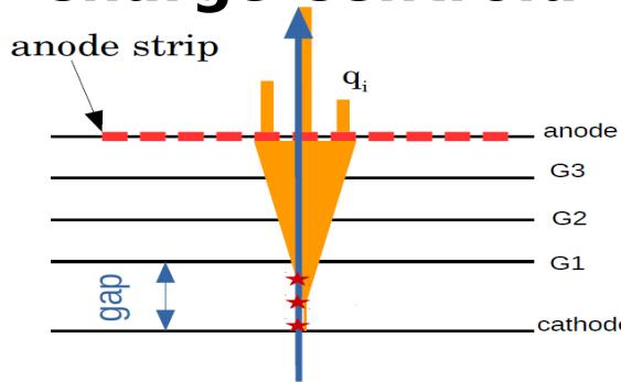
The position is reconstructed as weighted average of the fired strips by the charge on each strip
