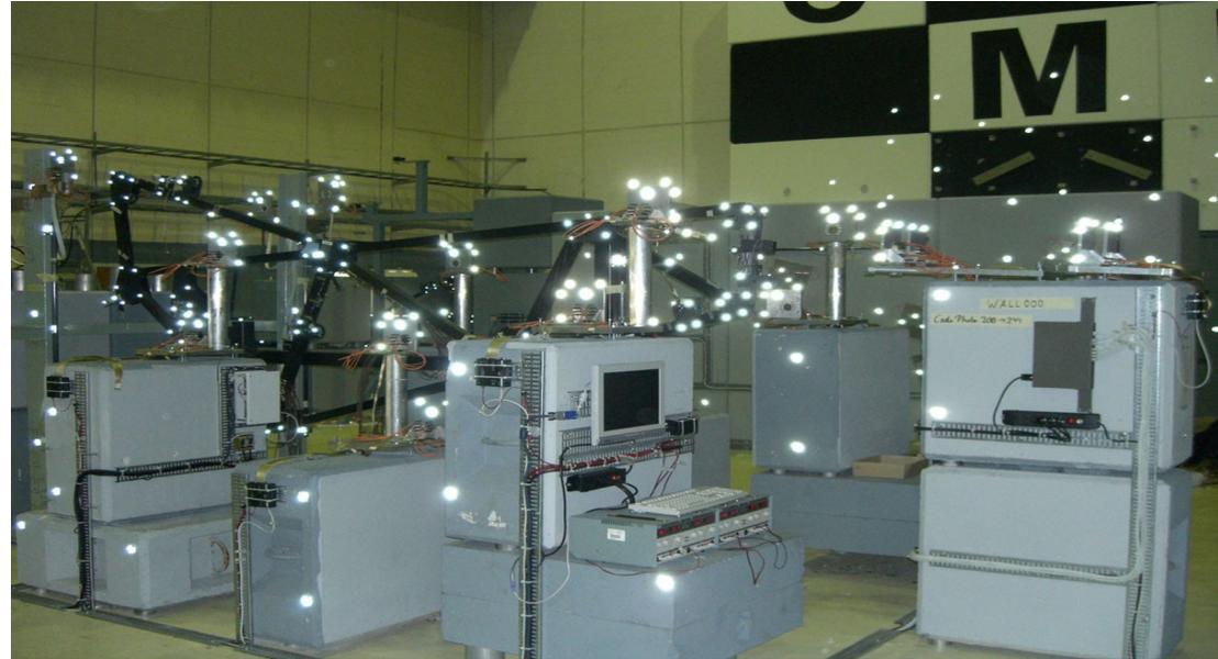
**Photogrammetry is used also to calibrate the hardware alignment systems**
