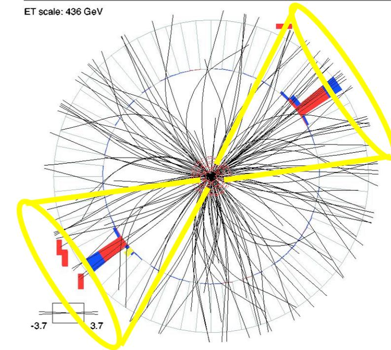
Jets are defined in the central region using seed-based cone algorithm (MidPoint - R=0.7)
