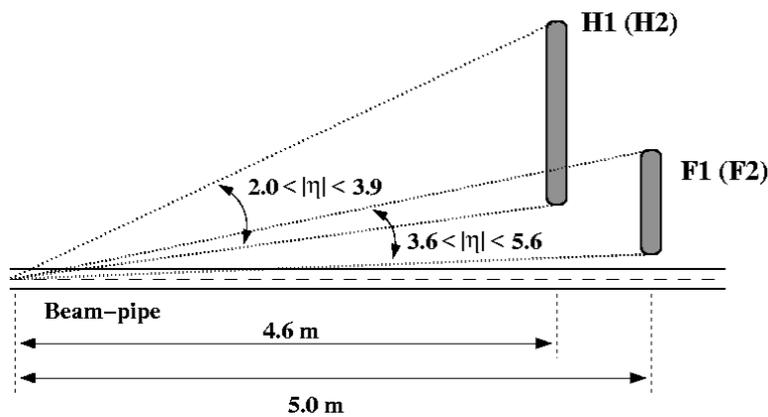
Require coincidence between beam crossing and at least one hit in each side of the trigger system.
