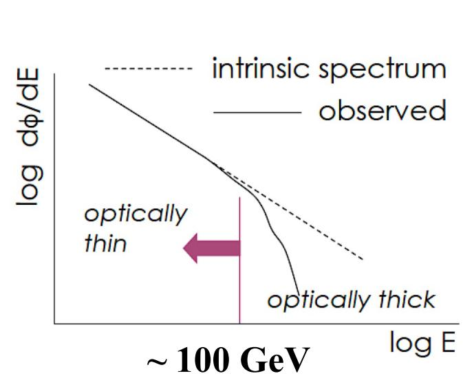
$$\left( \frac{d\phi}{dE} \right)_{\text{observed}} = \left( \frac{d\phi}{dE} \right)_{\text{intrinsic}} e^{-\tau(E,z)}$$
